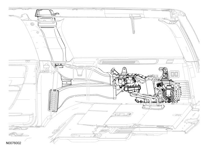
The auxiliary heater core and evaporator core housing is located behind the passenger side lower quarter trim panel. Do not mount any equipment to the housing. Do not mount any equipment in a way that may block the air intake or vents.
